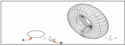
Select the object to revolve (A) and the axis (B) about which to revolve it. followed by the angle of revolution.
