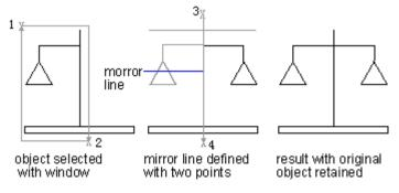
System variable MIRRTEXT affects texts created with MIRROR command. When MIRRTEXT is on, the copy of text object is displayed in mirroring way as other objects do. When MIRRTEXT is off, the direction of text objects remains unchanged. Displaying as follows:
