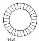
If you select a closed polylines, the ruled surface begins at the last vertex and proceeds backward along the polyline segments. If you select open curves, selecting objects at the same side of the two objects to create ruled surface, selecting objects at different side of the two objects to create crossed ruled surface, shown as follows:
