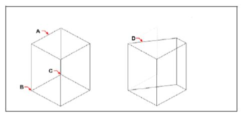
Specify the face(s) to taper ( $\mathbf{A}$ ), a The resulting entity with the face tapered to base point( $\mathbf{B}$ ), a second point position( $\mathbf{D}$ ). along the taper axis( $\mathbf{C}$ ), and a taper angle.
