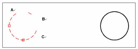
To scale using grips, select the object (**A**), click a grip (**B**), and Result. scale the object by dragging the grip to its new location (**C**).
