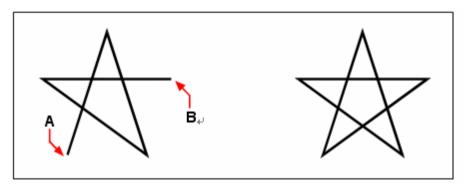
Closing an open polyline adds a straight polyline segment between the first (A) and last (B) vertices.
