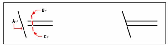
Select the boundary edge (A), and then specify the first point (B) and second point (C) of the fence.
