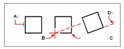
To rotate an entity in reference to a base angle, select the entity (**A**), specify base point (**B**), select the reference angle and pick point (**B**) again (or type the @ symbol), specify the second point (**C**), and then specify the point representing the new angle (**D**).
