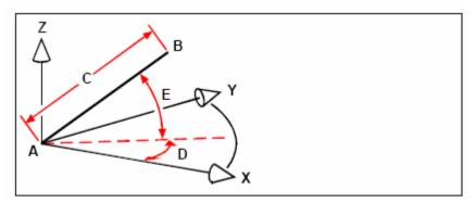
When you draw a line from a start point (**A**) to an endpoint (**B**) using spherical coordinates, you specify its length (**C**, in this case 10.2500 units), the angle in the xy plane (**D**, in this case 45 degrees), and the angle from the xy plane (**E**, in this case 35 degrees).
