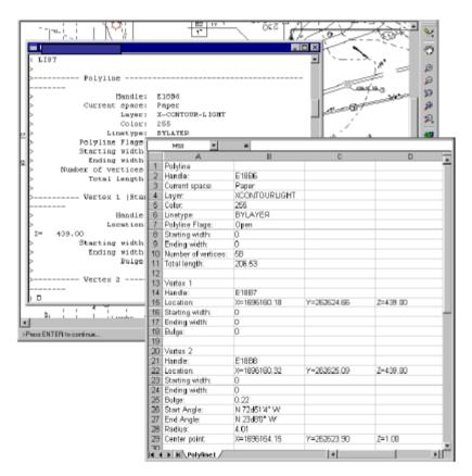
You can extract information stored in the drawing as visible or invisible attributes and use that data for analysis in a database or spreadsheet.
