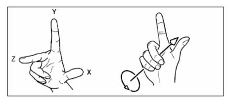
The right hand rule helps you determine the positive direction of the x, y, and z axes and the positive rotation direction.
