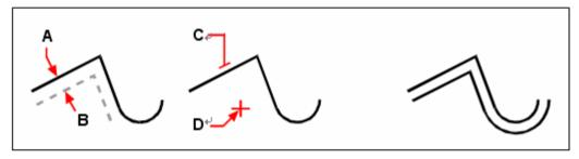
To make a parallel copy, specify the distance between copies Result. by entering a distance or selecting two points (A and B), select the object to copy (**C**), and specify on which side to place the copy (**D**).
