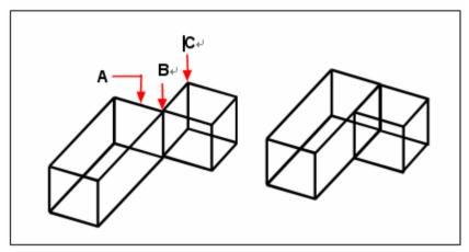
Specify the face(s) to move(A), the The resulting object with the face base point (B), and the end point moved to the new position.
