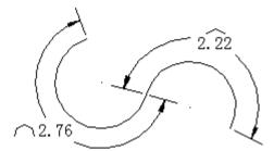
Additionally, orthogonal or radial extension line is available for arc length dimension, only the included angle of the arc segment selected for creating arc length dimension is smaller than 90 degree can display it's orthogonal extension line.
