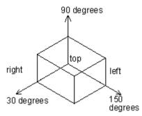
In addition to using ISOPLANE command to switch isometric planes, you can also use shortcut key F5 or CTRL+E. specifying one of the three isometric planes results in Ortho and crosshairs to be aligned along the corresponding isometric axes.
