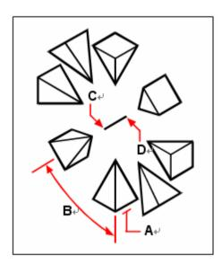
To create a three dimensional polar array, select the object to copy (**A**), type the number of items to array, specify the angle the array is to fill (**B**), and then specify the center point of the array (**C**) and a second point along the central axis of the array (**D**).
