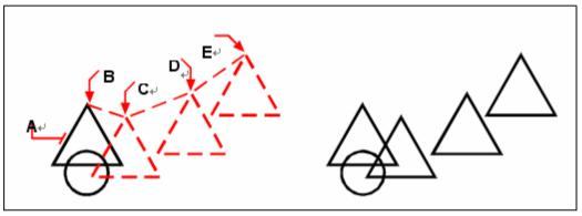
To make multiple copies of an object, select the object to copy (A), specify the base point (B), and then specify the displacement points (C, D, and E).
