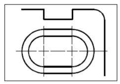
Snap and entity snap force the cursor to adhere to a specified increment or attach to key geometric points on existing entities. You can also constrain lines to vertical and horizontal axes.
