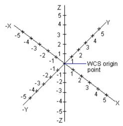
Generally, the WCS and the UCS are coincident with each other, which means that their axes and origin points are overlapped exactly. No matter how many times you relocate the UCS, you can always use the World option of the UCS command to make it coincident with the WCS.
