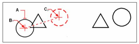
To move an object, select it (A), and then specify the Result base point (B) and the displacement point (C).
