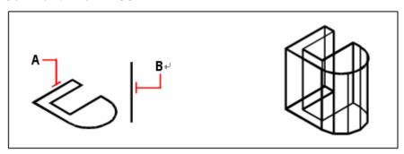
Select the object to extrude (A) and The resulting extruded surface mesh. the extrusion path (B).
