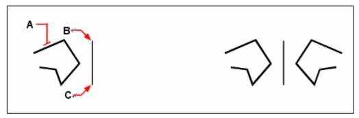
To mirror an object, select it (**A**), and then specify the first point (**B**) and second point (**C**) of the mirror line.
