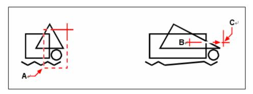
To stretch objects, select them using a crossing window (**A**) or crossing polygon, and then specify the base point (**B**) and displacement point (**C**).
