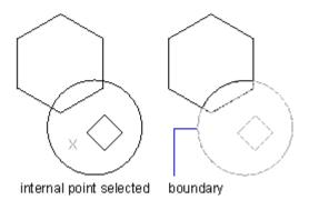
With the Boundary command, you can designate a specific area of a drawing for operations such as hatching and dimensioning. You create a boundary polyline by selecting an area inside a closed loop. The area you select can be bounded by a single closed object or by multiple objects that intersect.
