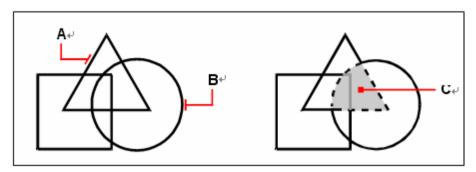
Selected objects (**A** and **B**). which results in a new boundary around the shaded area.
