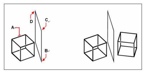
Select the object to mirror (**A**), and then specify the first point (**B**), second point (**C**), and third point (**D**) defining the mirror plane.
