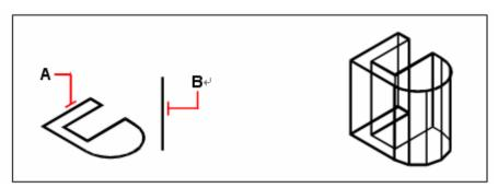
Select the object to extrude (A) and the The resulting extruded surface mesh. extrusion Path (B).
