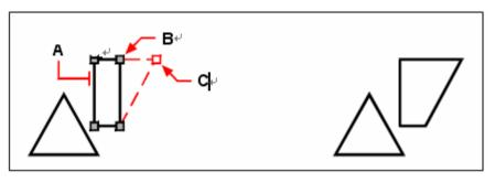
To stretch an object using grips, select the object (A), select a grip (B), and drag the grip to its new location (C).
