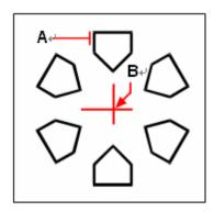
To create a polar array, select the object to copy (A), specify the center point of the array (B), and then specify the number of items to array, the angle the array is to fill, and whether to rotate the items.
