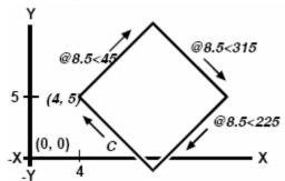
Drawing a tilted square using the relative polar coordinates method; enter *C* to close. **NOTE** This example, like all examples in this guide, assumes the program's default settings: Angles increase counterclockwise and decrease clockwise. Thus, an angle of
