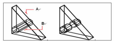
Select the objects to combine (A and B). The resulting combined solid. Use SUBTRACT to remove the common area of one set of solids from another.
