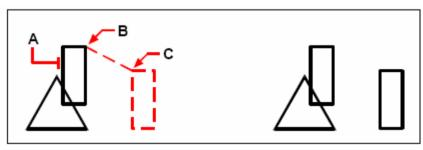
Object to copy (A), base point (B), and displacement point (C).
