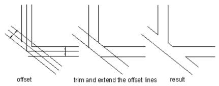
If the objects to offset are 2D polyline or spline, the system trims them automatically when the specified distance is larger than can otherwise be accommodated. Displaying as follows:
