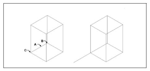
Specify the edge(s) to copy (A), the The resulting entity with the edge base point (B), and the end copied. point(C).
