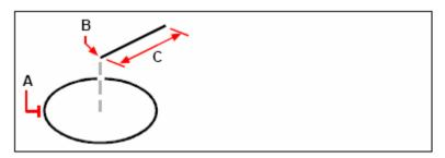
You can use point filters to draw a line by first selecting a point in the xy plane (A), specifying the z coordinate (B), and then specifying the length of the line (C).
