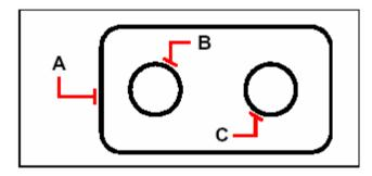
To calculate the area of the gasket using the Area command, first add the area of the entire gasket (A), and then subtract the areas of the two circles (B and C). As you select objects, the program displays the calculations. If the command bar is displayed, the information appears there. If the command bar is not displayed, the
