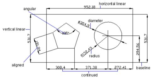
When you create a dimension, the program draws it on the current layer, using the current dimension style. Each dimension has an associated dimension style, which controls the appearance of the dimension, such as the types of arrowheads, text style, and colors of various components. You can modify existing dimension styles by changing any of the dimension variable settings, and the new dimension style is visible soon after you confirm the modification.
