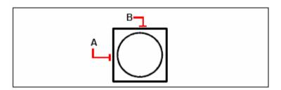
You can use point filters to center the circle by separately selecting the midpoints of two sides of the rectangle (A and B) and then specifying its radius.
