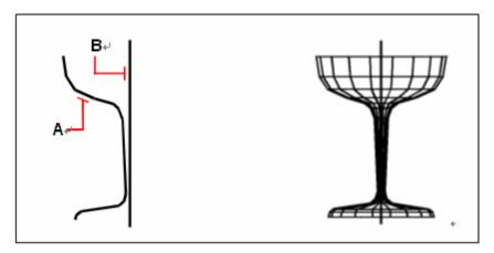
Select the object to be revolved (**A**) and the The resulting revolved surface mesh. axis of revolution (**B**).
