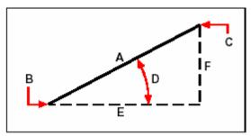
Use the Distance command to calculate the distance (A) between two points (B and C), the angle in the xy plane (**D**), the angle from the xy plane, and the delta x (**E**), delta y (**F**), and delta z distances between the two points.
