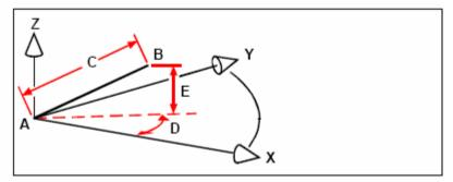
When you draw a line from a start point (**A**) to an endpoint (**B**) using cylindrical coordinates, you specify its length (**C**, in this case 7.4750), the angle in the xy plane (**D**, in this case 27 degrees), and the distance in the z direction (**E**, in this case 3 units).
