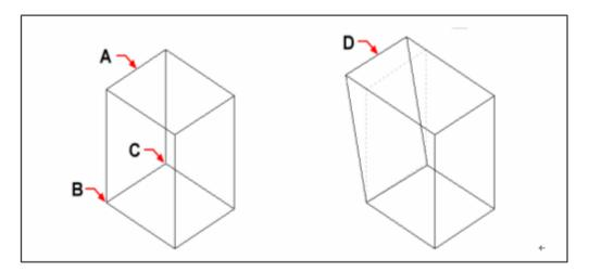
Specify the face(s) to rotate (A), the base point (B), a second point on tapered the rotation axis (C), and a rotation angle.
