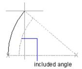
The included angle determines the endpoint of the arc. Use the Start, End, Angle method when you know both endpoints but cannot snap to a center point.
