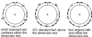
The justification and other settings may affect the vertical alignment of text. If you select Horizontal Alignment, text inside the extension lines and centered within the dimension is placed horizontally, as shown in the leftmost figure above.
