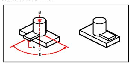
Select the objects to rotate (**A**), specify the endpoints of the axis of rotation (**B** and **C**), and then
