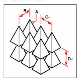
To create a three dimensional rectangular array, select the object to copy (**A**), type the number of rows, columns, and levels, and then specify the distance between each row (**B**), column (**C**), and level (**D**).
