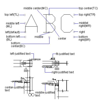
You can also align text so that it fits or aligns between two points. The Align option creates text that scales up or down while maintaining a constant height/width ratio; the Fit option expands or compresses the text to fit between the two points.
