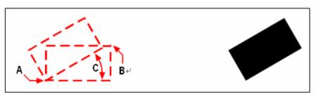
Opposite corners (A and B) and rotation angle (C). Resulting plane.
