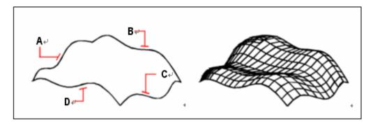
Select the objects to be used as the four The resulting Coons surface patch mesh. edges (**A**, **B**, **C**, and **D**).
