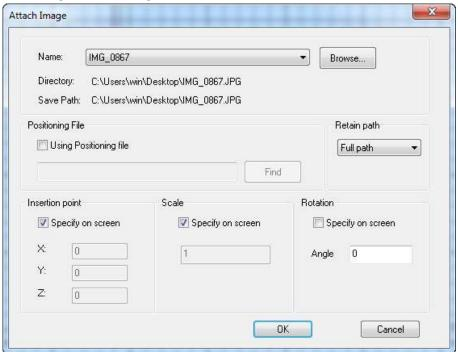
You can also attach raster image by Image Manager, inputting command IMAGE to open the Image Manager Dialog box, click Attach button to browse raster image, specify the insertion scale, position and rotation angle in the dialog box. With Image Manager dialog box, you can also detach, reload, unload or save the path of the raster image.
